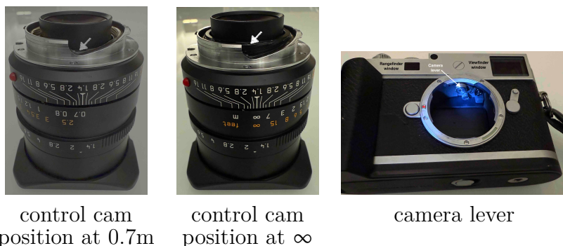
Figure 12: Mechanical link between the lens focus and camera
