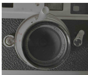
incorrectly mounted lens (lever on the right)
